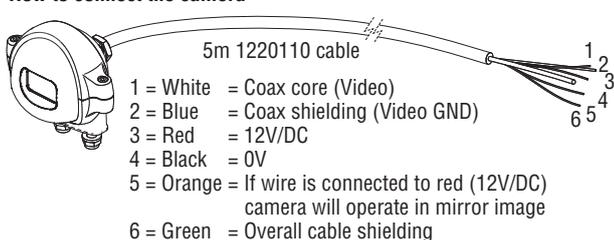
**NOTE:** The free end of the permanently connected, unterminated cable is to be connected in an appropriate way, e.g. with the Orlaco Junction box Ex.
