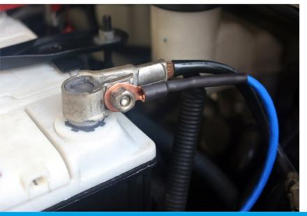
Example of installation on Lead Acid battery terminal. The sensor terminal lug can be easily attached to the terminal post and will conduct the temperature directly to the sensor chip.
