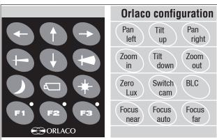
To switch to the ORLACO configuration, press and hold the Tilt up button and the F1 button for 1 second during start up the keyboard. (BLC = Back light compensation)
