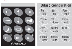
To switch to the ORLACO configuration, press and hold the Tilt up button and the F1 button for 1 second during start up the keyboard. (BLC = Back light compensation)
